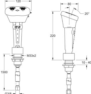
**NOVALAB** eye shower for wall mounting on laboratory furniture with stainless steel braided pressure hose and wall bracket witrh wall duct; with DVGW type examination certificate
