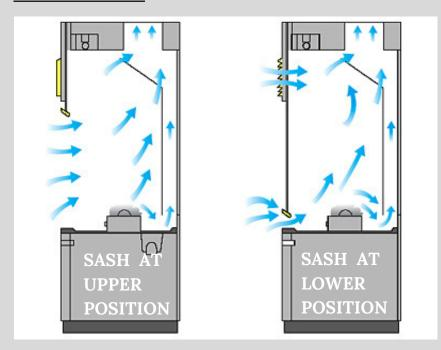
The bypass system allows air flow even while the sash is closed. This provides constant air volume regardless of sash position. The air bypass provides for an alternate route for air to enter the hood if the sash is closed.
