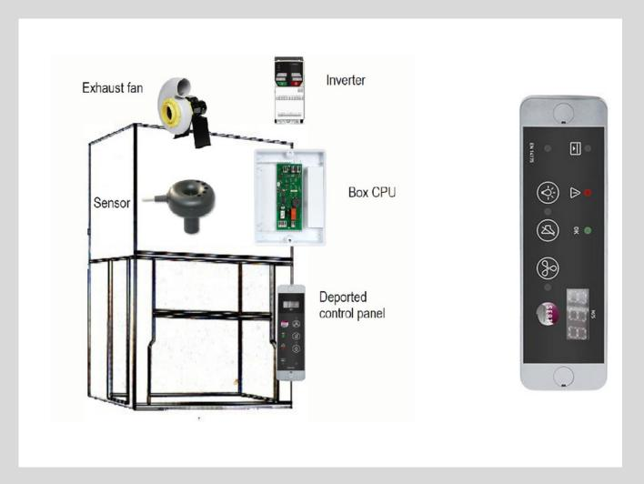
Equipped with variable airflow controller
