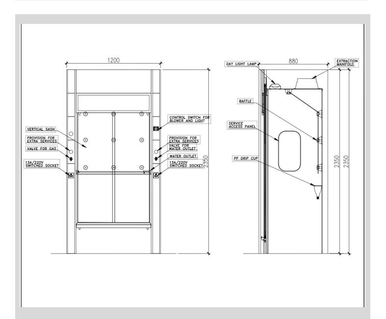
Walk-in fume cupboard is appropriate for placing large floor standing equipments.
