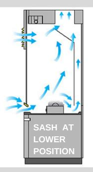
The bypass system allows air flow even while the sash is closed. This provides constant air volume regardless of sash position. The air bypass provides for an alternate route for air to enter the hood if the sash is closed.
